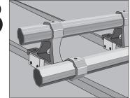
For maximum holding strength, setscrews should be tensioned and re-tensioned as the seam material compresses. Screw tension should be verified using a calibrated torque wrench between 160 and 180 inch pounds when used on 22ga steel and between 130 and 150 inch pounds for all other metals and thinner gauges of steel.
